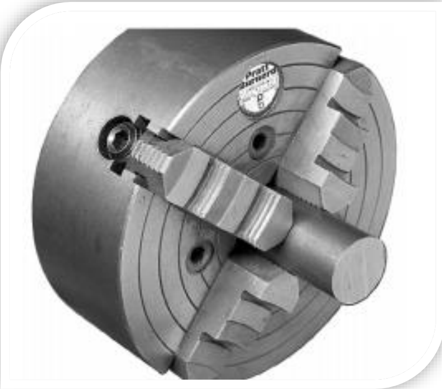
Four-jaw independent chuck.
