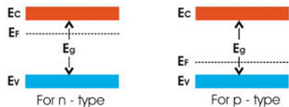
Figure 9.2: Fermi Level in Extrinsic semiconductors
